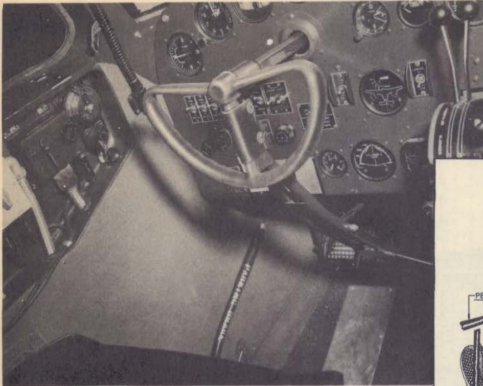
Figure 19 - Installation of Controls Lock
